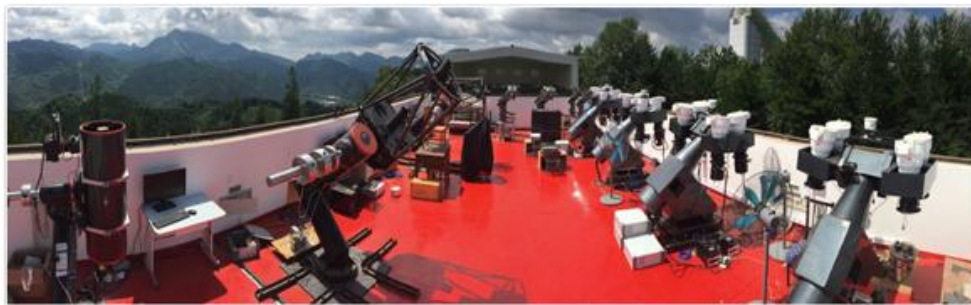
Fig2. GWAC and its follow-up telescope, including two 60 cm telescopes and one 30 cm telescope. Currently, all these are set at Xinglong station, NAOC, China,
