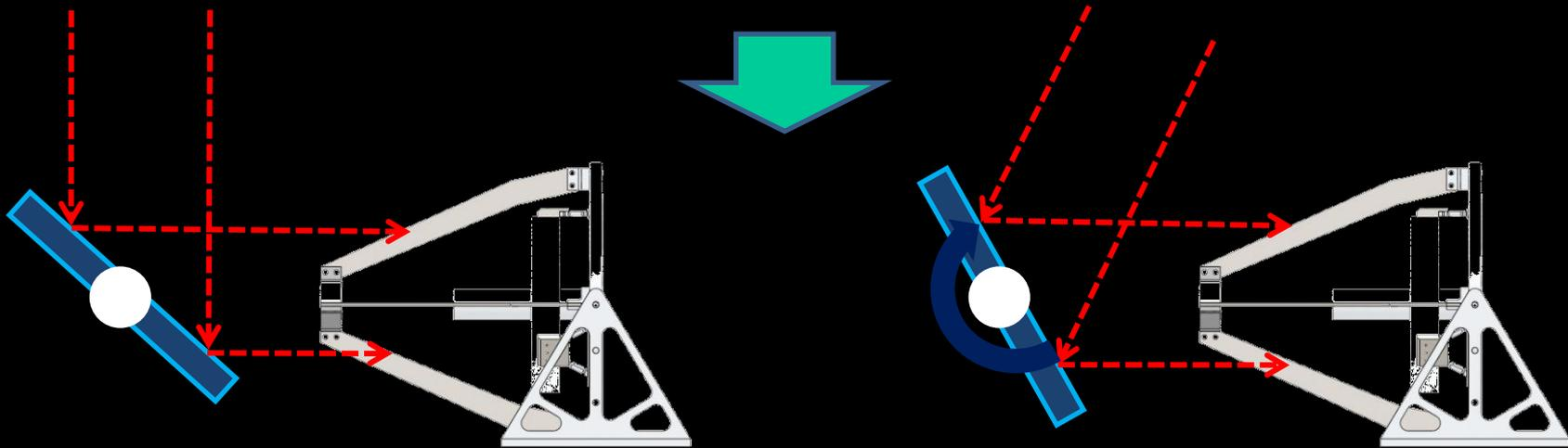
In UFFO-p, we move the optical path, not the spacecraft with fast slewing mirror system → much faster (~3 s, NEW Concept)
