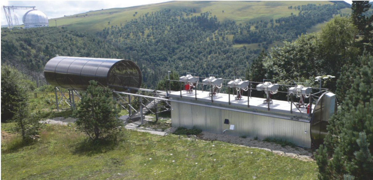
Fig2. Photo of the all 9 channels of MMT installed on 5 mounts in the single cylindrical dome, which is open at that moment. Russian 6-m telescope may be seen in the background.
